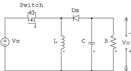
Fig. 1. Circuit of Buck-Boost Converter
