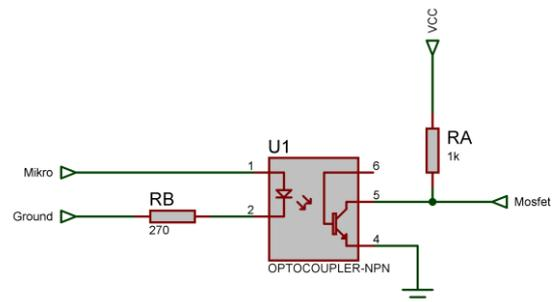
Fig. 7. MOSFET Driver Circuit
