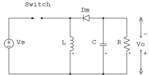
Fig. 3. Buck-Boost Converter With Switch On
