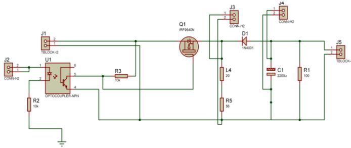
Fig. 8. Circuit of Converter Buck Boost
