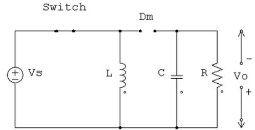
Fig. 2. Buck-Boost Converter With Switch Off
