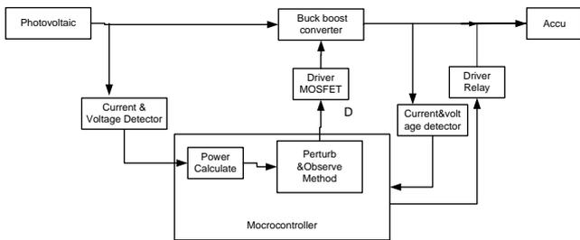
Fig. 6. Diagram Block of MPPT For Photovoltaic
