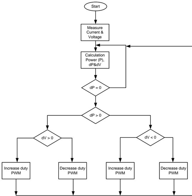
Fig. 5. Flowchart of Perturb and Observe Method
