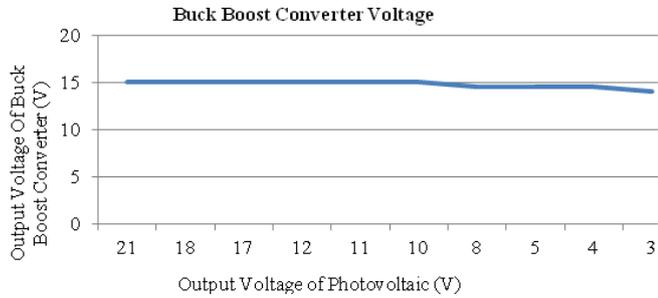
Fig. 10. Buck Boost Converter Voltage To Photovoltaic Output Voltage
