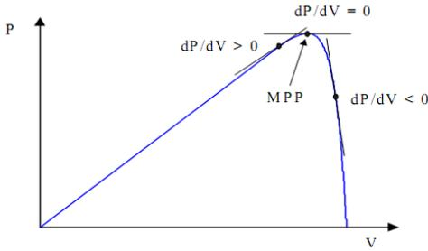
Fig. 4. Curve of Maximum Point Tracking
