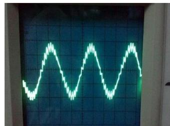
Fig. 9. Inverter Output with Frequency switching 1000 Hz
