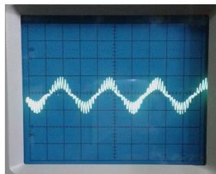
Fig. 10. Inverter Output with Frequency switching 4000 Hz
