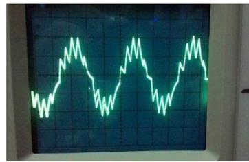
Fig. 8. Inverter Output with Frequency switching 500 Hz
