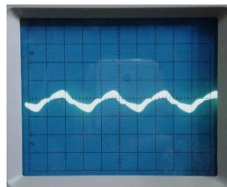
Fig. 11. Inverter Output with Frequency switching 10000 Hz
