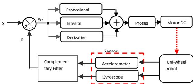
Fig. 3. Uni Wheel Diagram block
