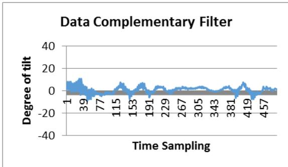
Fig. 15. Complementary Filter response when the robot maintain a balance with a load of 48 kg
