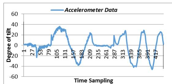
Fig. 7. Tilt angle measurement data with ADXL345 accelerometer sensor
