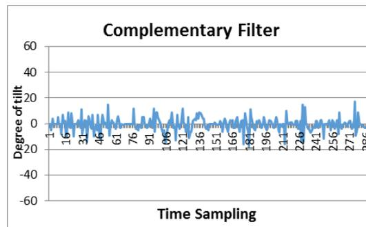
Fig. 12. IMU sensor for  $k_p=600$ ,  $K_i=10$  and  $K_d=10$
