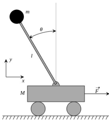
Fig. 1. Inverted pendulum robot movement.
