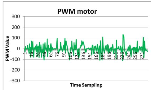
Fig. 13. PWM response for  $k_p=600$ ,  $K_i=10$  and  $K_d=10$
