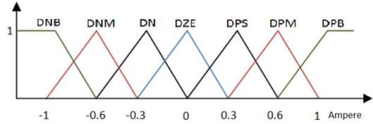
Fig. 10 – Membership function of input delta error
