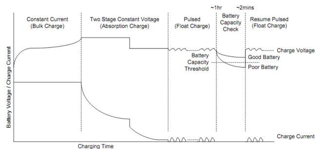
Fig.5 – The characteristic of charging method of SLA battery [9].
