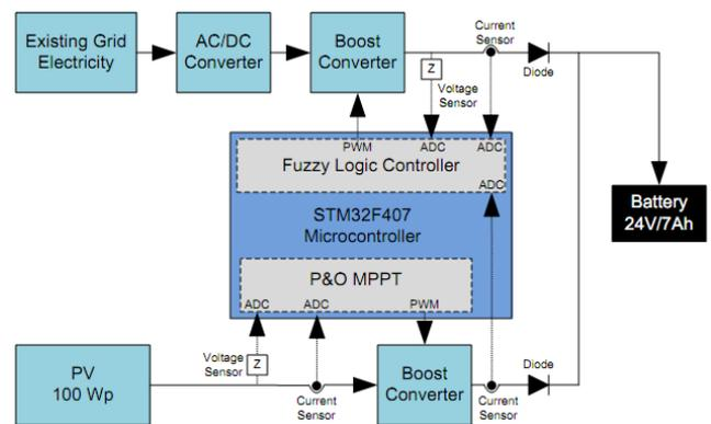
Fig.6 – General block diagram for proposing hybrid battery charging system.
