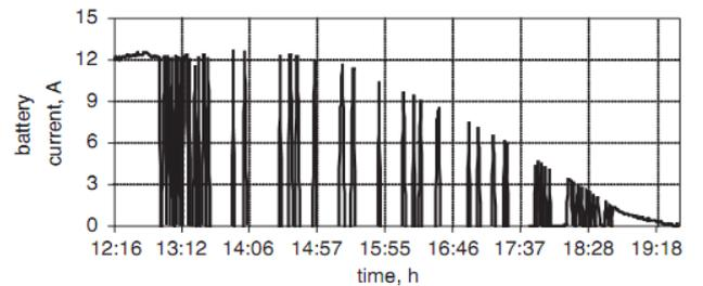
Fig.4 – Characteristic of Standalone PV for battery charging [6].
