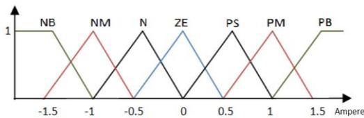
Fig. 9 – Membership function of input error
