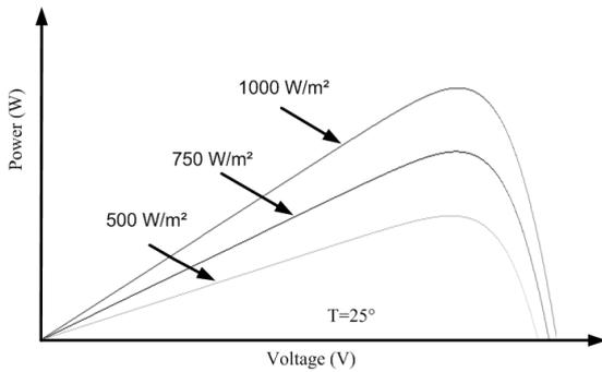
Fig. 1. Influence of the solar irradiance for constant temperature
