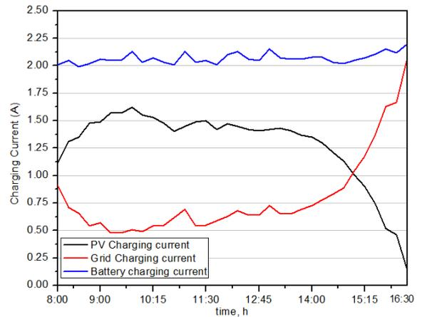
Fig.15 – Result of hybrid battery charging with load sharing algorithm.
