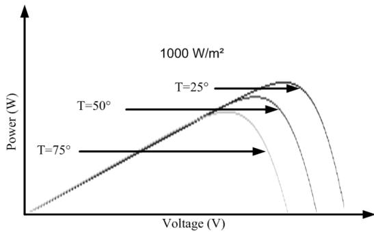
Fig. 2. Influence of the solar temperature for constant irradiance
