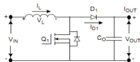
Fig. 7 – Boost converter and its signal of operation
