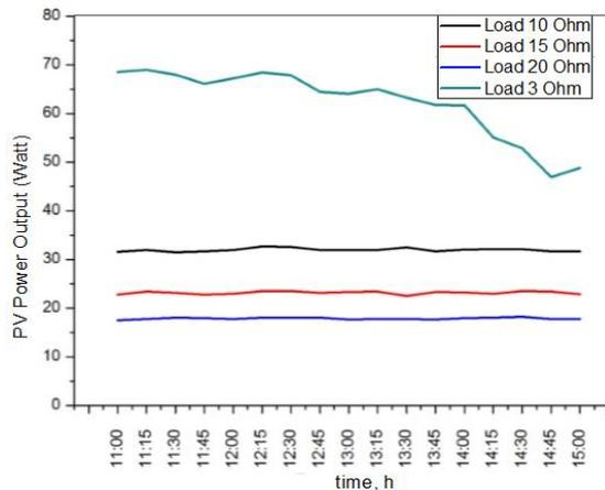
Fig. 13. Hourly characteristic of PV power output without MPPT.
