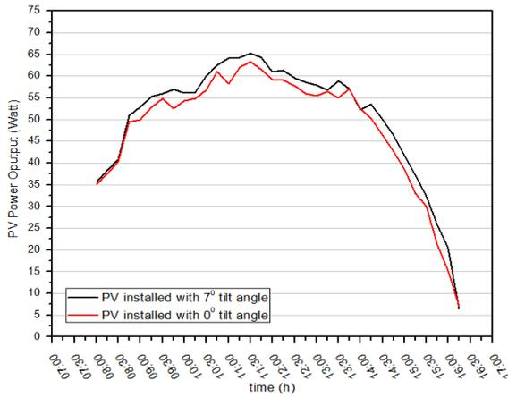
Fig. 12. Hourly characteristic of PV power output.
