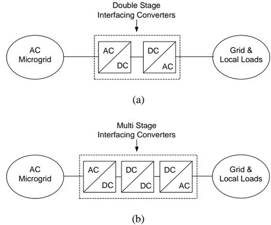
Fig. 3. Power electronic interfaces for microgrid with ac output powers (a) Double stage ac-dc and dc-ac interfacing converter (b) Multi stage ac-dc, dc-dc and dc-ac interfacing converter
