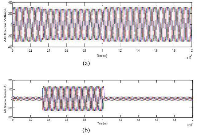
Fig. 9. AC Source (a) Voltage (b) Current
