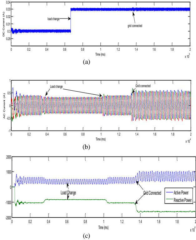
Fig. 7. Connected by bidirectional converter and grid (a) DC current (b) AC current (c) AC power
