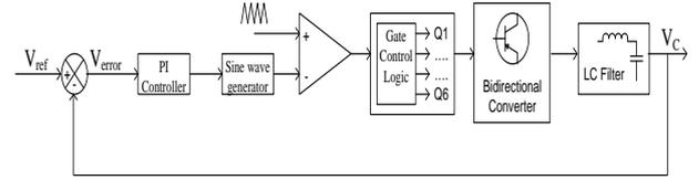
Fig. 5. Basic block diagram of the voltage control method
