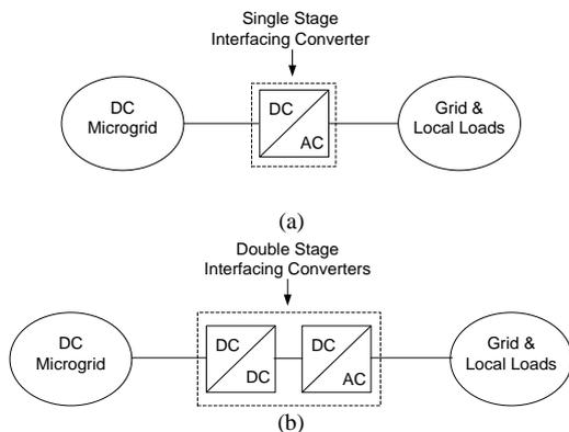
Fig. 2. Power electronic interfaces for microgrid with dc output powers (a) Single stage dc-ac interfacing converter (b) Double stage dc-dc and dc-ac interfacing converter
