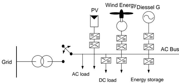
Fig. 1. Distributed AC bus architecture of hybrid microgrid
