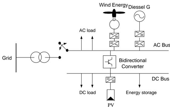
Fig. 4. Distributed AC – DC bus architecture of hibrid microgrid
