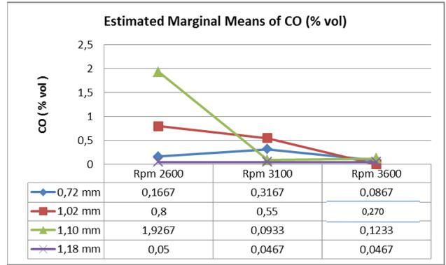
Fig. 3. Variation chart Size Hole Diameter Main Jet against CO (% volume)
