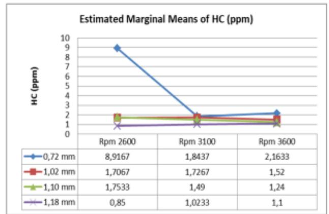
Fig. 4. Variation chart Size Hole Diameter Main Jet against HC (ppm)
