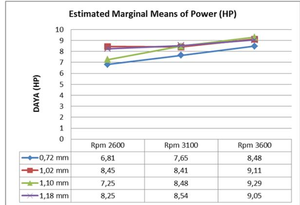
Fig. 2. Diameter Hole Size chart Variations of the Main Jet Power
